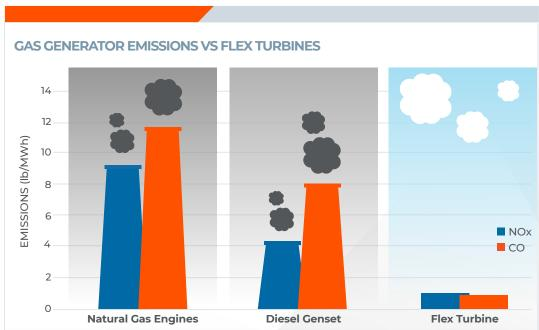
While some diesel gensets emit less than comparable natural gas engines, the transfer of diesel fuel to power them drives the total emissions to significantly higher levels. Meanwhile, Flex Turbines meet the California Air Resources Board Distributed Generation Standard when operating on pipeline natural gas with our integrated cogeneration heat exchanger.
